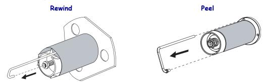
**3.** Slide the media liner off of the spindle and discard.
